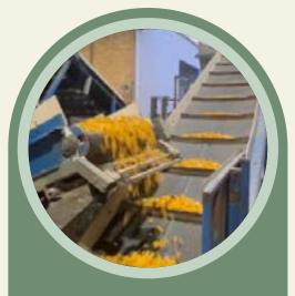
The granulator breaks down the old chairs into recyclable plastic pellets, ready to be moulded into new chairs.
